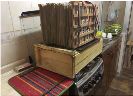
Fig. 2. Herbarium press placed on a gas stove to benefit from passive convectional heating.
