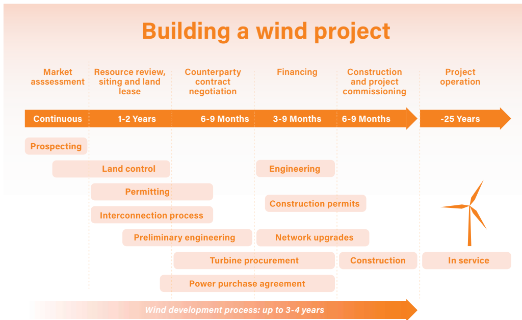
Figure 1: Onshore wind development process. Source: Wind Exchange, 2024
